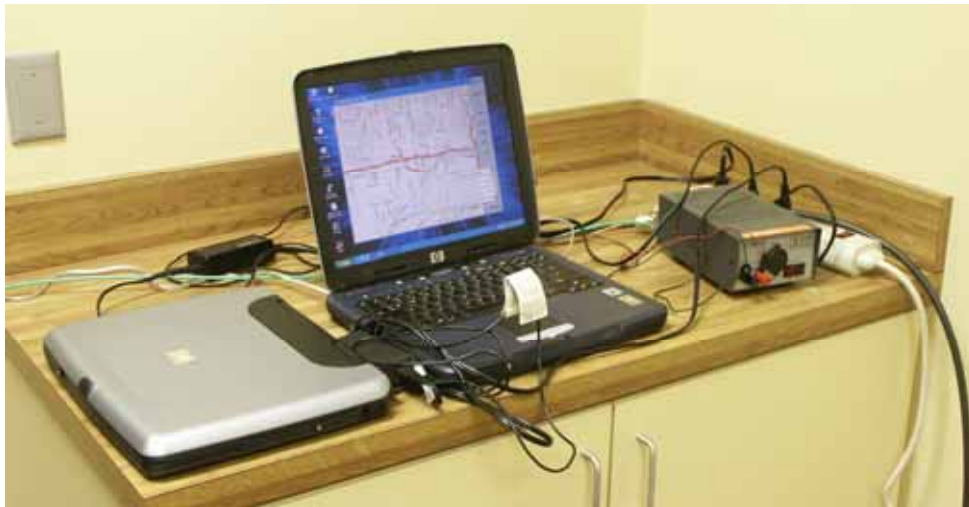
Figure 1. Central System Controller (CSC) for test application.
