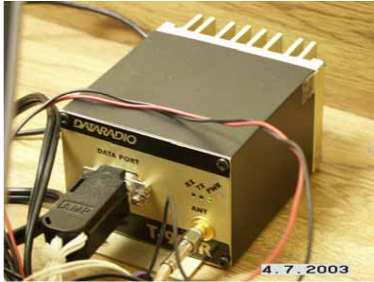
Figure 2. Data modem used by CSC to communication with field components.\
