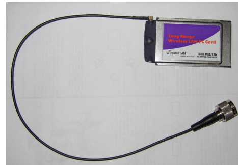
Fig. 10. Senao NL-2511CD PLUS EXT2 wireless network interface card. The antenna pigtail and connector are also shown.
