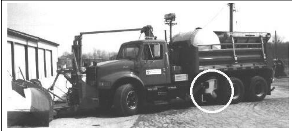
Figure 8-2 Friction meter, Iowa prototype vehicle
