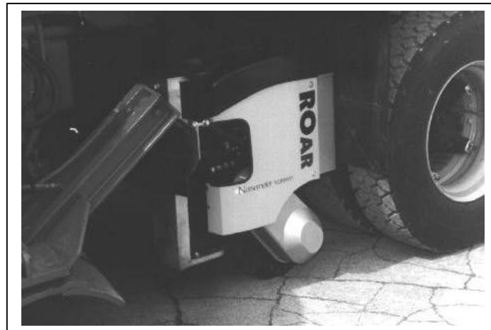
Figure 8-3 Friction meter, Iowa prototype vehicle
