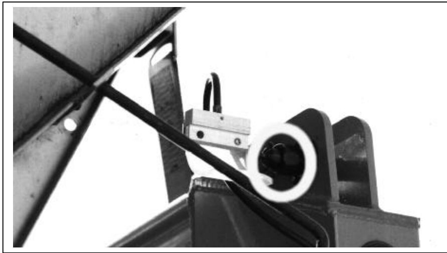
Figure 11-3 Right ball-and-socket joint (circled), HID lighting system, Iowa vehicle
