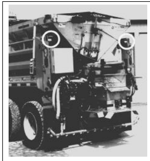
Figure 11-1 Fiber optic light system (circled), Iowa prototype vehicle
