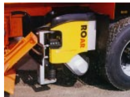
pavement friction measuring device Roadware Corporation Ontario Canada and Norsemeter Company Rud, Norway
