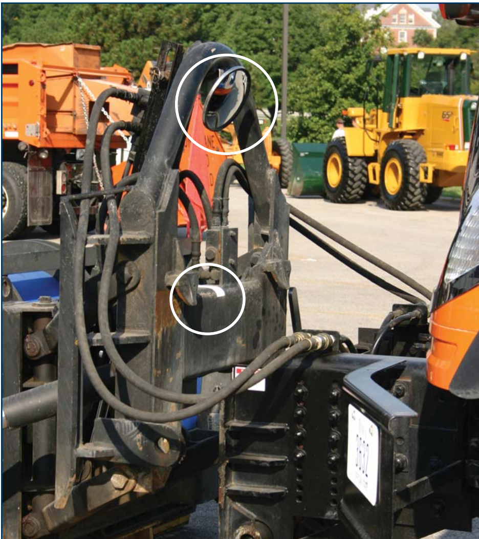
A mirror and some silver tape make it easier for a driver to load a plow alone.
