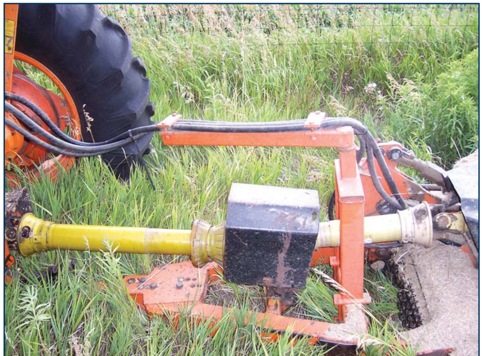
Extend the life of hydraulic hoses with the organizer.
