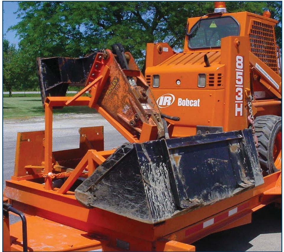
The attachment rack is attached to the same trailer that the skid loader rides.
