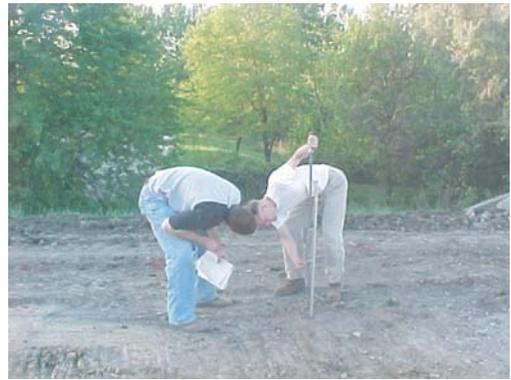
*Dynamic cone penetrometer testing*
