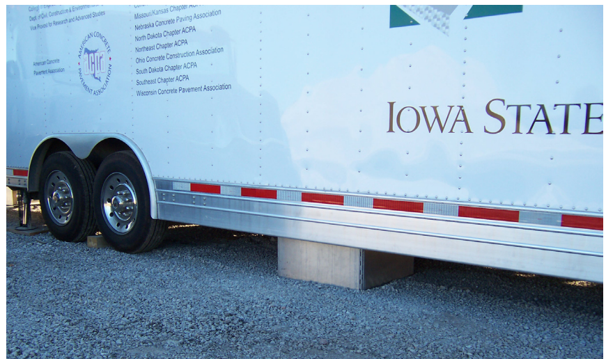
View of the weather shield from the exterior of the CP Tech Center Mobile Concrete Research Lab
