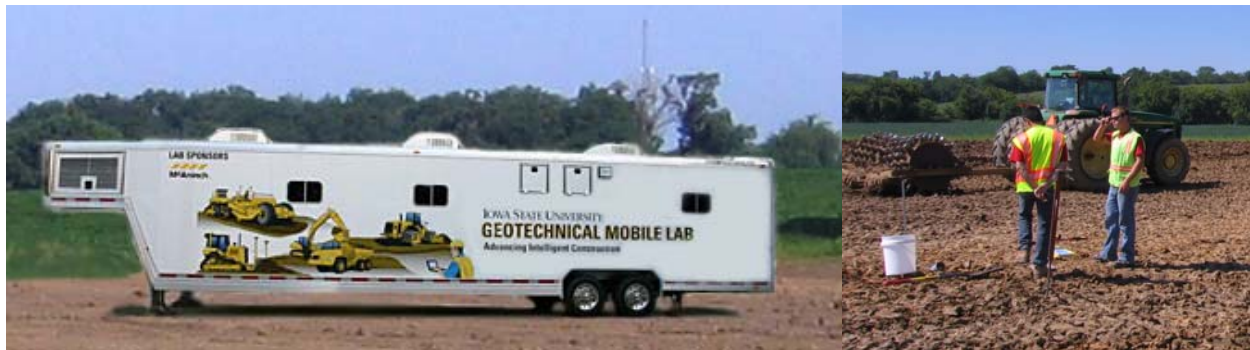
Figure 8. Geotechnical Mobile Lab (left) and Iowa State University Q/A testing at the Crow Creek embankment on August 17, 2006 (right)
