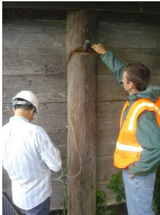
**Figure 3. Pile integrity testing (Bridge No. 237350, Mahaska County)**
