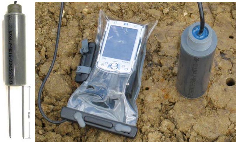
Figure 2. IMKO TRIME-EZ probe (left) and inserted into soil (right) with TRIME Data Pilot
