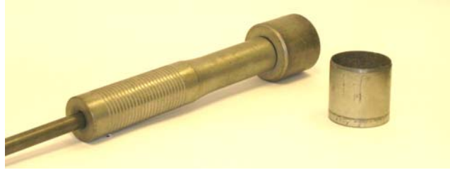
Figure 5. Drive core sampling device
