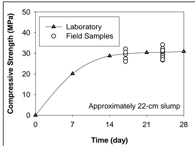
**Figure 2. Grout maturity curve and pile compressive strengths**
