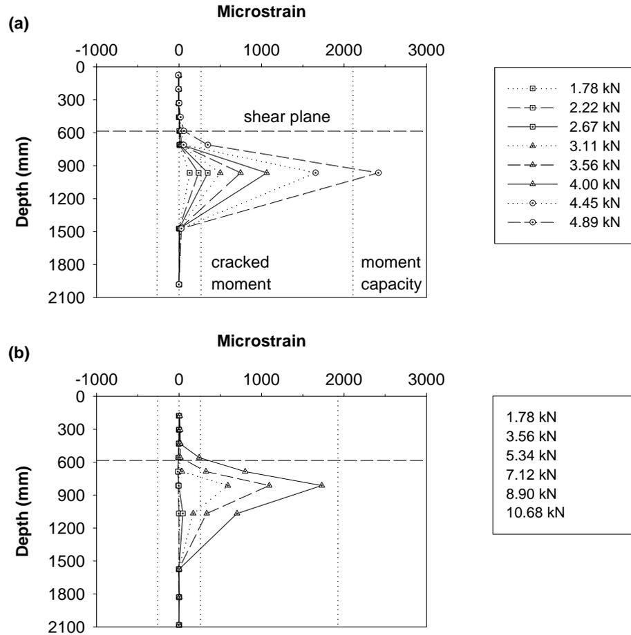
**Figure 9. Strain profiles for piles in loess**
