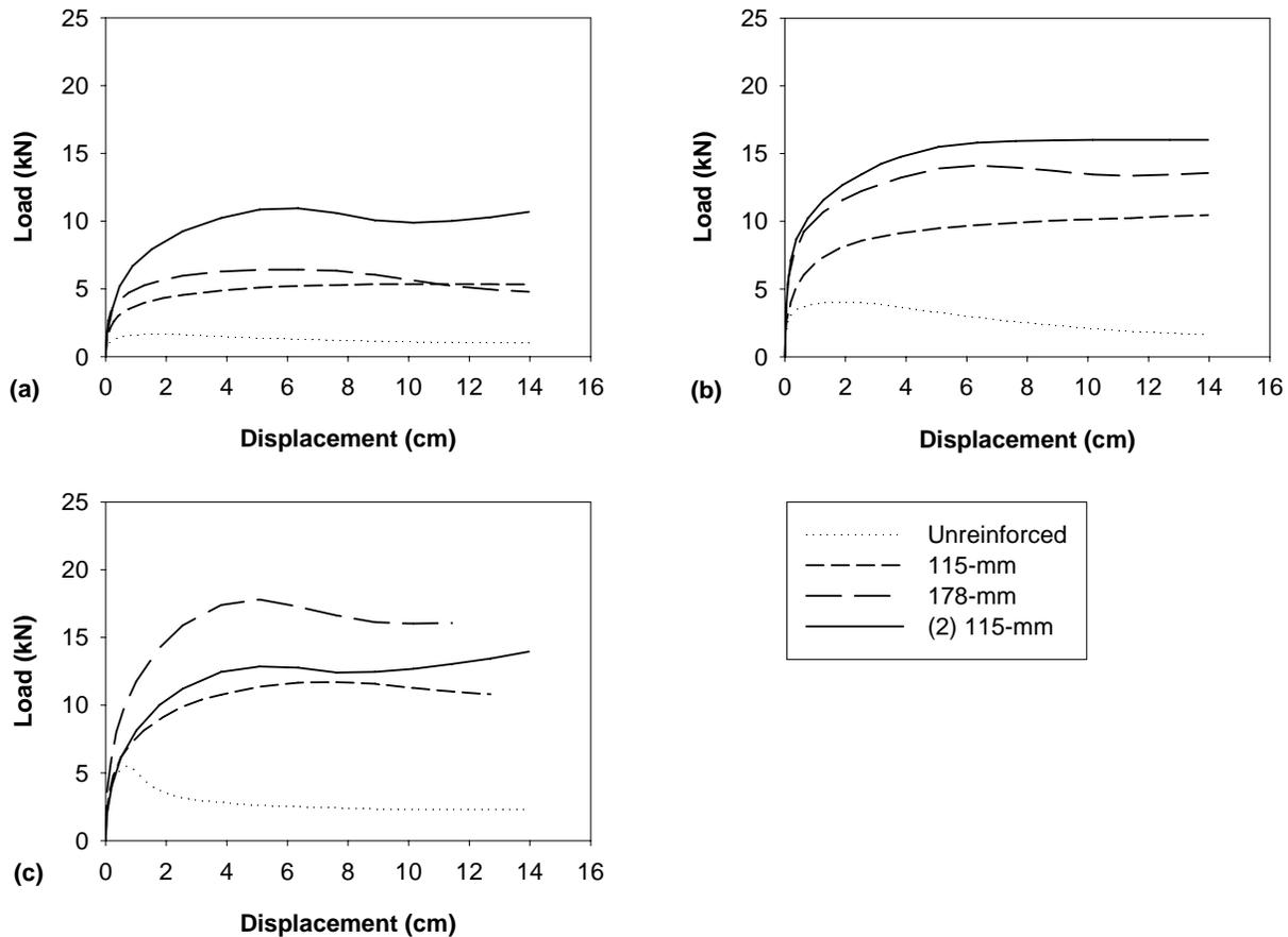
**Figure 3. Load-displacement relationships**
