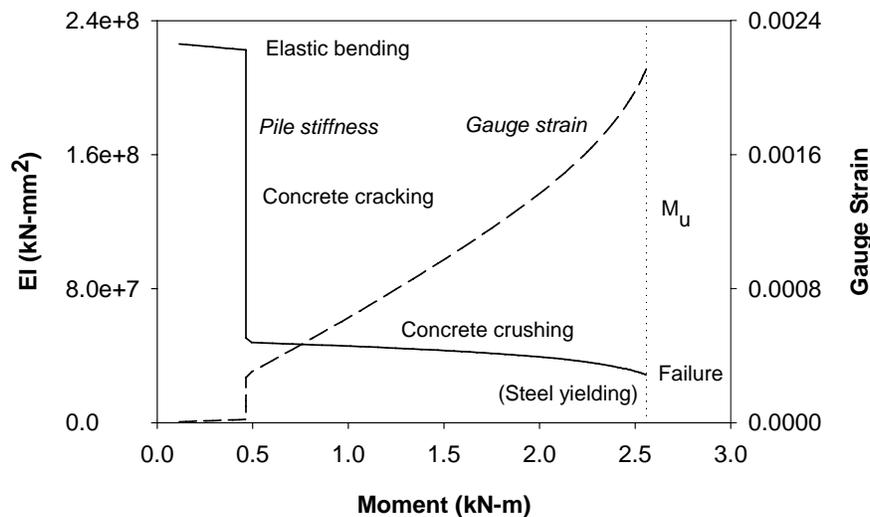
**Figure 8. Flexural stiffness gauge strain-bending moment relationship**
