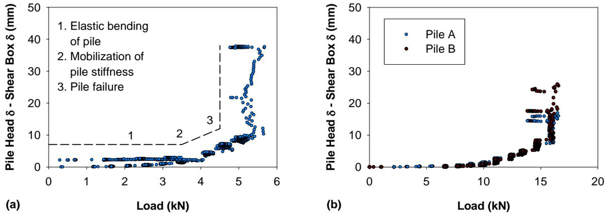
**Figure 4. Behavioral stages of piles subject to lateral soil movement**
