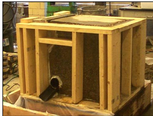
**Figure 9. Using porous fill material behind the abutment**
