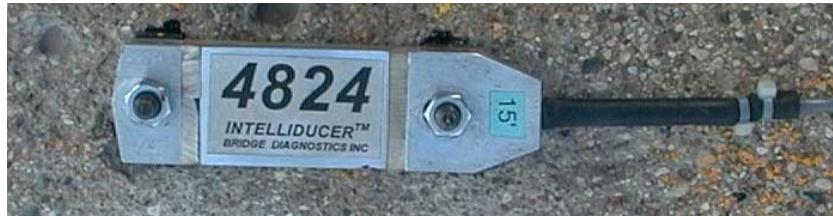
FIGURE 1. A BDI Intelliducer in Use on Top of a Concrete Curb
