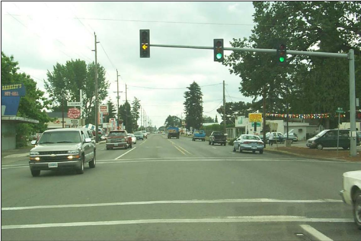
**FIGURE 5. Four-Section Vertical Flashing Yellow Arrow Permissive Indication**
