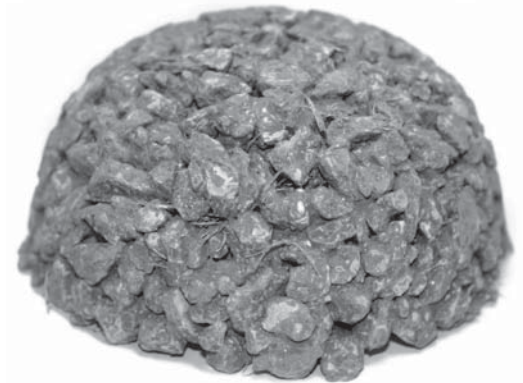
Figure 1. A "popcorn ball" textured sample of pervious concrete.
