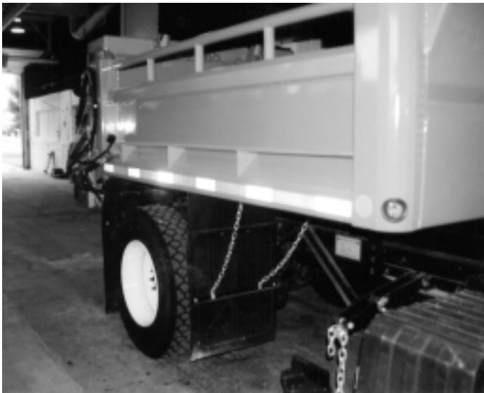
The camera's flash had the effect of light from headlamps on retro-reflective tape installed on the sides and rear of this vehicle.
