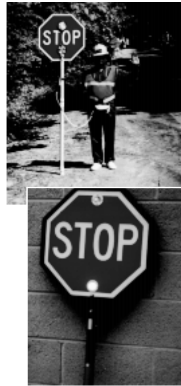
Flashing stop/slow paddles grab drivers' attention more effectively than conventional paddles. Photos courtesy of Peter Hatzi, Federal Highway Administration.
