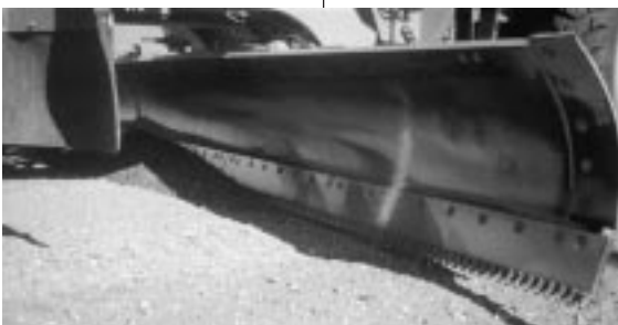
Rotating bits do a good job of smoothing a gravel road.
