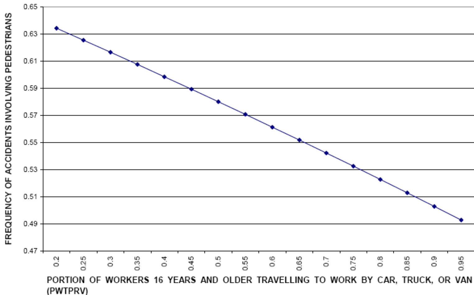
Exhibit 95: Predicted number of Crashes involving pedestrians by TAZ by portion of workers age 16 and older traveling to work by car, truck, or van, by TAZ:- PLANSAFE pedestrian model
