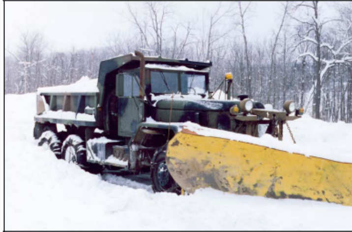
Figure 2. M34 2-1/2-ton, 6 × 6 dump truck manufactured by the Reo Truck Company in 1952–53 mounting a cable/hydraulic Roadway model 1d single-blade non-reversible 12-foot snowplow. The plow was manufactured in the 1963–66 time frame and is still in use today.
