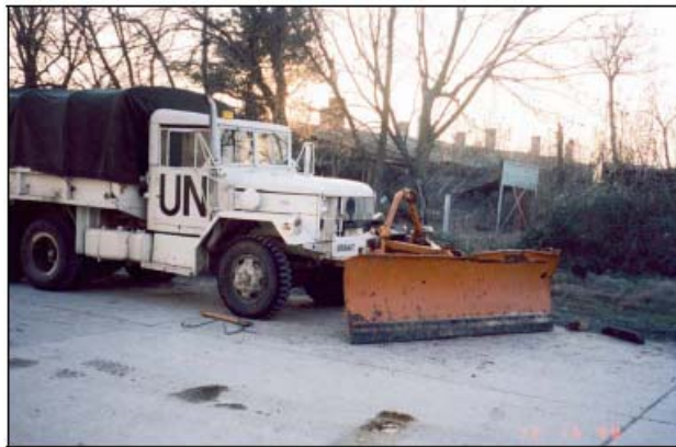
Figure 3. 1966 M35 6 × 6, 2-1/2-ton truck mounted with an early German-built Schmidt Engineering 11-foot conventional, manually reversible snowplow manufactured in 1950. This plow was in service in Baumholder, Germany, with the U.S. Army for 43 years before being shipped to Task Force Able Sentry in 1994, where it continues in service today.
