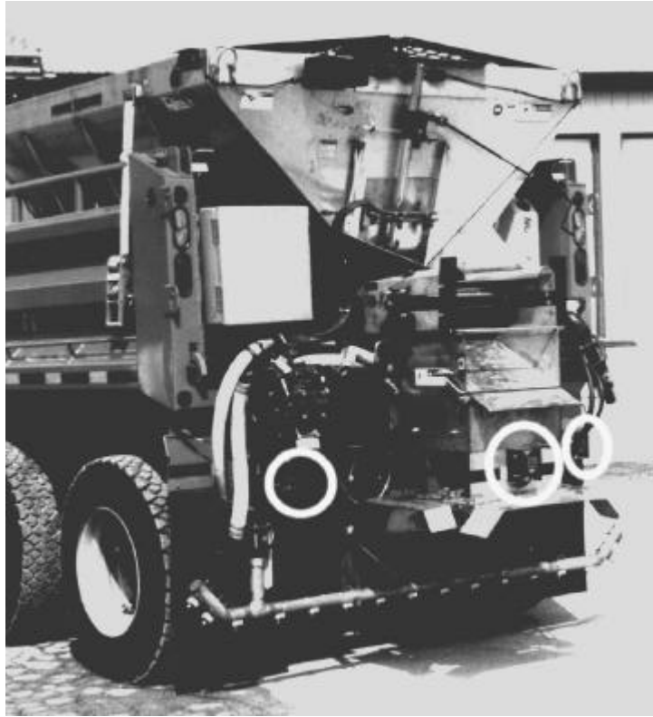
Figure 12-1 Location of reverse obstacle sensors (circled), Iowa vehicle
