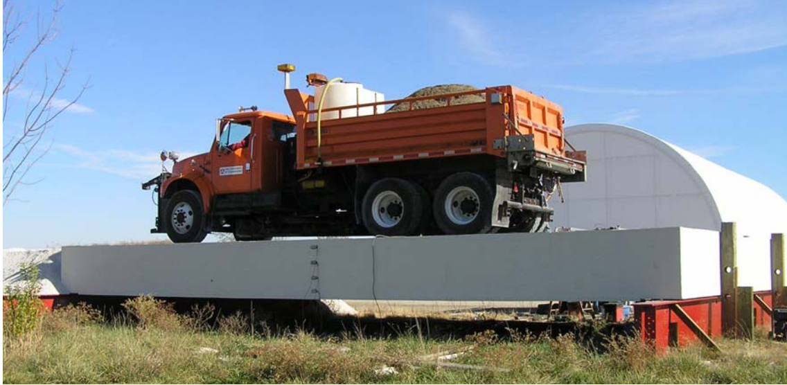
Figure 1. Bridge on temporary supports subjected to test load
