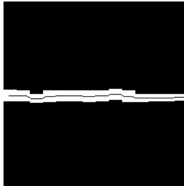
Figure 13. Visualization of crack shape and area and thinned line used for length calculation
