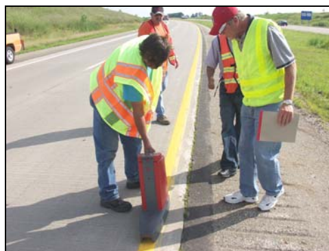
Figure 7. Handheld Delta LTL-X machine
