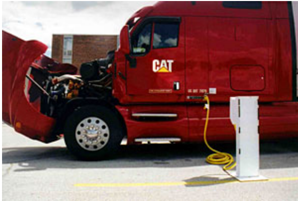
CAT MorElectric truck with ShurPower hook-up.
