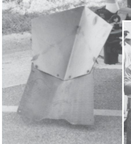
The stainless steel and rubber reciprocating chute spreads salt more evenly on the road.
